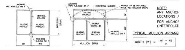
Mull span and tributary width are first calculated as shown in the above sketch. One would then enter the non-reinforced (06-0620.18) product approval with this information, and determine from the first (mull capacity) table which mull size would carry the applied pressure.
