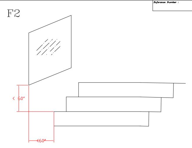
Glazing adjacent to a stairway within 60" horizontally of a bottom tread of the stairway in any direction, when the exposed surface of the glass is less than 60" above the nose of the tread. (2406.11)
