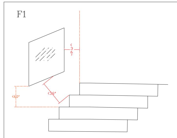
Glazing adjacent to a stairway, ramp or landing within 36" of a walking surface, when the exposed surface of the glass is less than 60" above the plane of the adjacent walking surface. (2406.3.1.0)
