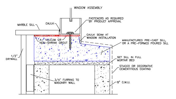
A — Any space existing between window's sill and precast sill will be filled with vulcum, or a non—shrink grout (not by window installer).
